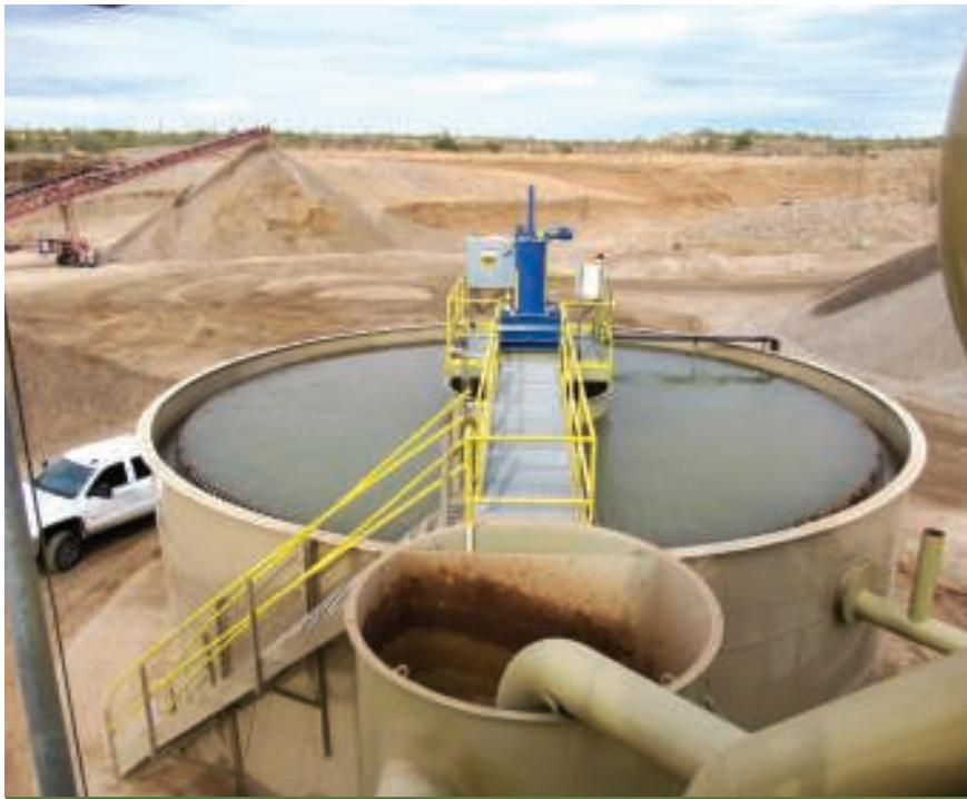
The 40-foot thickener tank allows the operation to reclaim and reuse up to 90 percent of the water from the wash plant.
