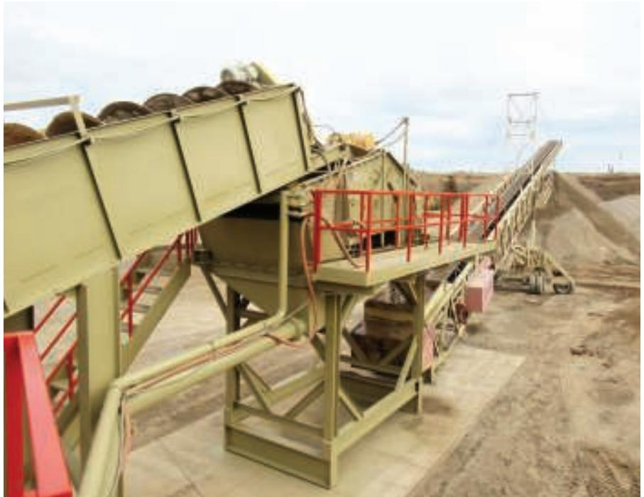
After leaving the attrition cells, sand travels through a sand screw and across the dewatering screen before being carried up the radial stacker to be stockpiled.
