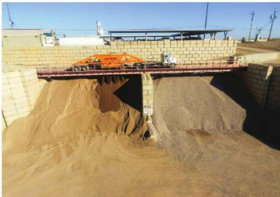
A belly-dump truck unloads material through a grizzly into the storage area of one of the ready-mix companies located on site at the Queen Creek operation.
